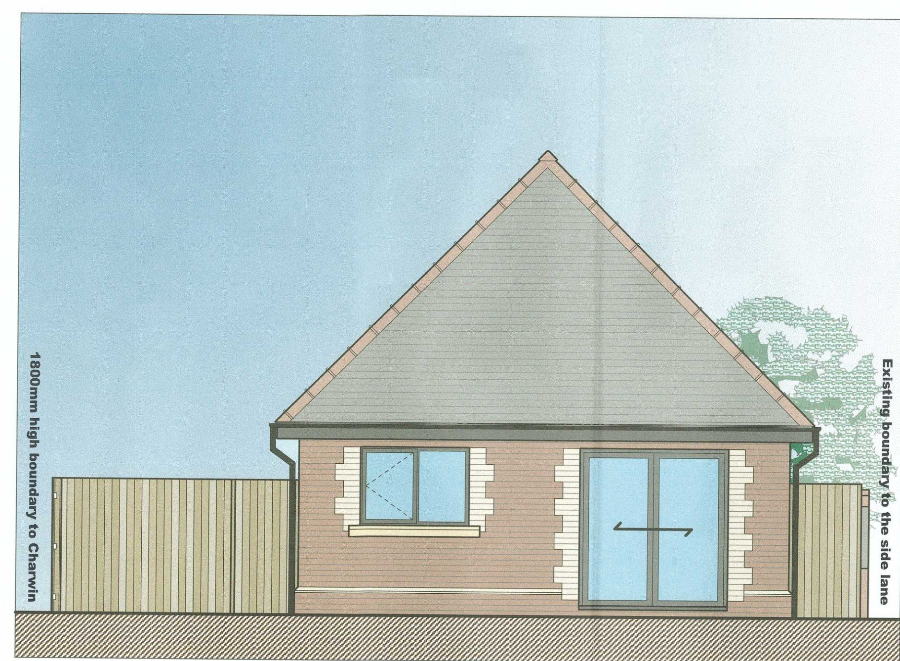
REAR ELEVATION EAST ELEVATION: SCALE 1 : 50 FACING THE GARDEN OF THE ADJOINING DWELLING
